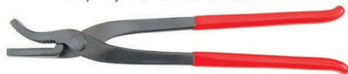
BRI-1-1104 Farrier Clincher For use with larger nails used in saddle horse hoofs to roll over and clinch nails. Oil quoting makes it rust resistant. Length 12" c/s. Also available in stainless steel.
