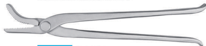
BRI-1-1102 Farrier Clincher For use on high and low nails. Used to roll over nails with curved jaw. Length 13" c/s. Also available in stainless steel.
